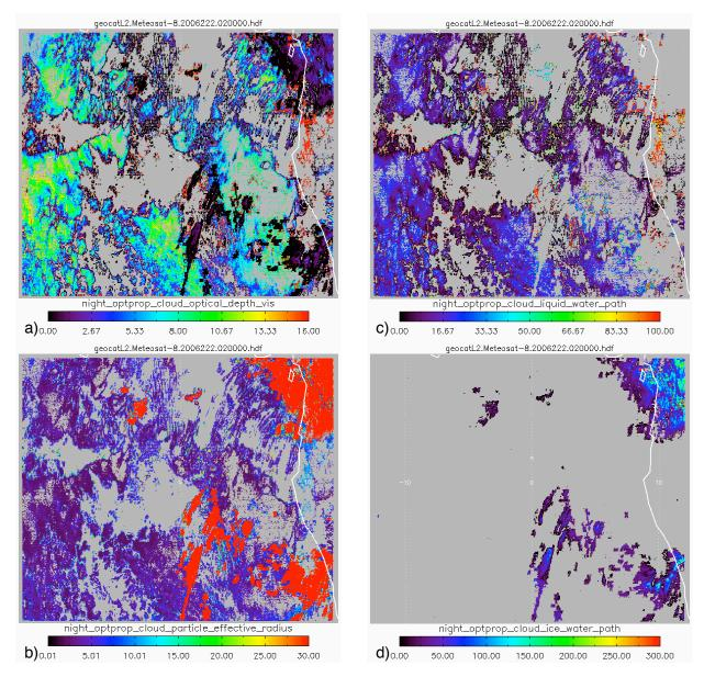
Figure 4. Results from 2 August 2006 0200 UTC. SIST utilized the input from Figs. 3 and 4 to obtain a) optical depth, b)  $r_e$  (microns), c) liquid water path (g/m<sup>2</sup>), and d) ice water path (g/m<sup>2</sup>).
