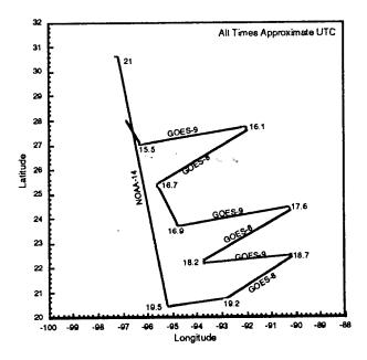
**Figure 2**. Flight path of ER-2 during second ARESE calibration flight. Legs corresponding to constant satellite viewing angle are indicated by the name of the satellite.
