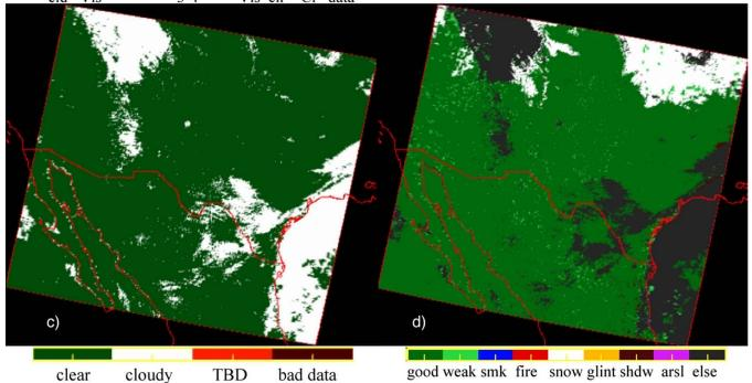
Fig. 13. Pixel classification by CERES daytime nonpolar cloud mask for Terra MODIS image in Fig. 12(a), 1700 UTC, December 21, 2000. (a) Final tests used to classify each pixel, (b) cloud quality classification, (c) final cloud mask, and (d) final clear-sky classifications.
