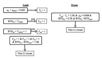
Fig. 8. Thin cirrus tests used for Aqua Ed1a processing after  ${\bf B}$  tests are applied.
