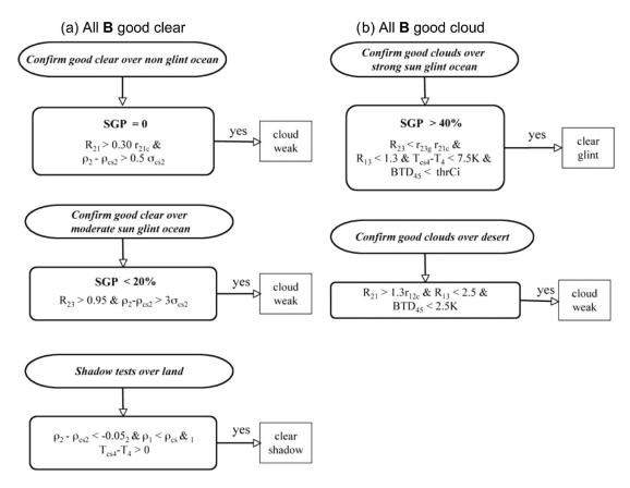
Fig. 7. Final classification for certain pixels classified as (a) clear or (b) cloudy after all of the **B** tests. If the specified conditions are met, the pixel is reclassified. SGP refers to sunglint probability.
