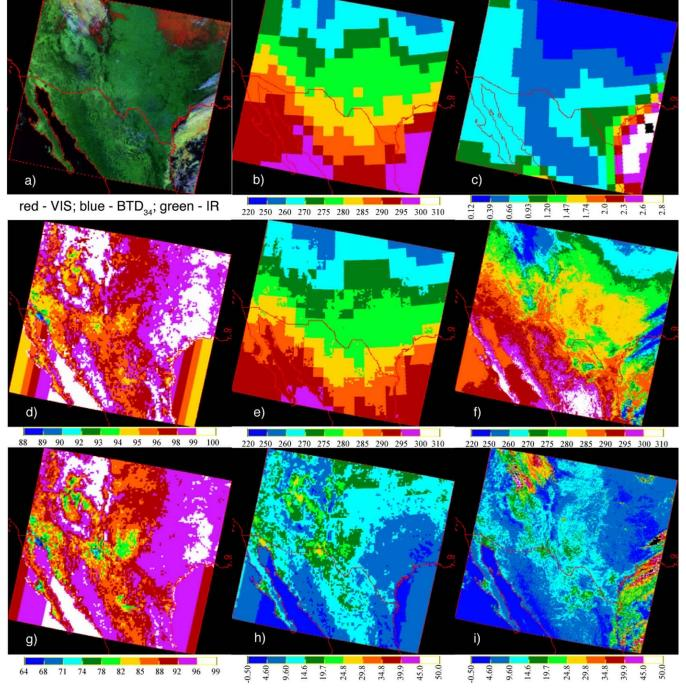
Fig. 12. Terra MODIS image, IR temperature, and BTD and mask input and predicted clear-sky IR and BTD parameters, 1700 UTC, December 21, 2000. (a) RGB image, (b) MOA skin temperature, (c) MOA precipitable water vapor in centimeters, (d) IR surface emissivity, (e) predicted clear-sky IR brightness temperature  $T_{cs4}$ , (f) observed IR brightness temperature, (g) 3.8- $\mu$ m surface emissivity, (h) predicted clear-sky BTD<sub>cs34</sub>, and (i) observed BTD<sub>34</sub>.
