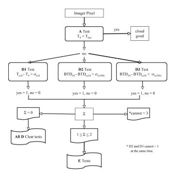
Fig. 14. Schematic diagram of CERES nonpolar nighttime scene identification.
