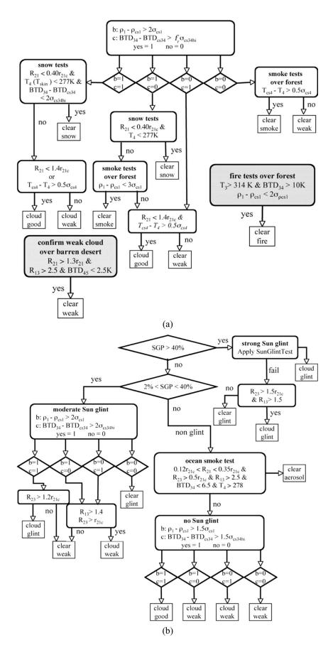
Fig. 9. (a) Daytime, C1 test over land. B1 = 0, B2 = 1, and B3 = 1. The relaxation factor  $f_r$  is 2.0 for desert and 1.5 for nondesert land. Parameters shown in italics indicate tests only used by Aqua Ed1. The  $T_{skin}$  test for b = 1 and c = 1 is only used for Terra Ed2. The free-floating tests are applied only to certain surface types after the C1 tests are completed. (b) Same as (a), except over ocean.
