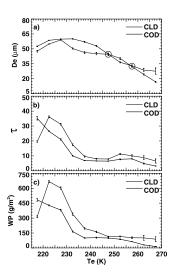
**Figure 3.** Comparison of the mean and standard error of the cloud properties over the CLD and COD regions as a function of  $T_e$  for (a)  $D_e$ , (b)  $\tau$ , and (c) WP. The vertical bars are the standard errors  $(\sigma/\sqrt{N})$ , where  $\sigma$  is the standard deviation and N is pixel number) for the CLD and COD regions, respectively. The two circled points indicate that the mean differences between CLD and COD are not significant.
