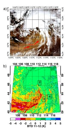
**Figure 1.** (a) The true color composite over Northwest China, in which three channels, 0.65, 0.56 and 0.47 $\mu$ m, are associated with red, green and blue colors, respectively. (b) The BT difference between 11 and 12  $\mu$ m channels (T45). Box 1 is the DUST region, box 2 the CLD region, box 3 the PCOD region, and box 4 the COD region, respectively.
